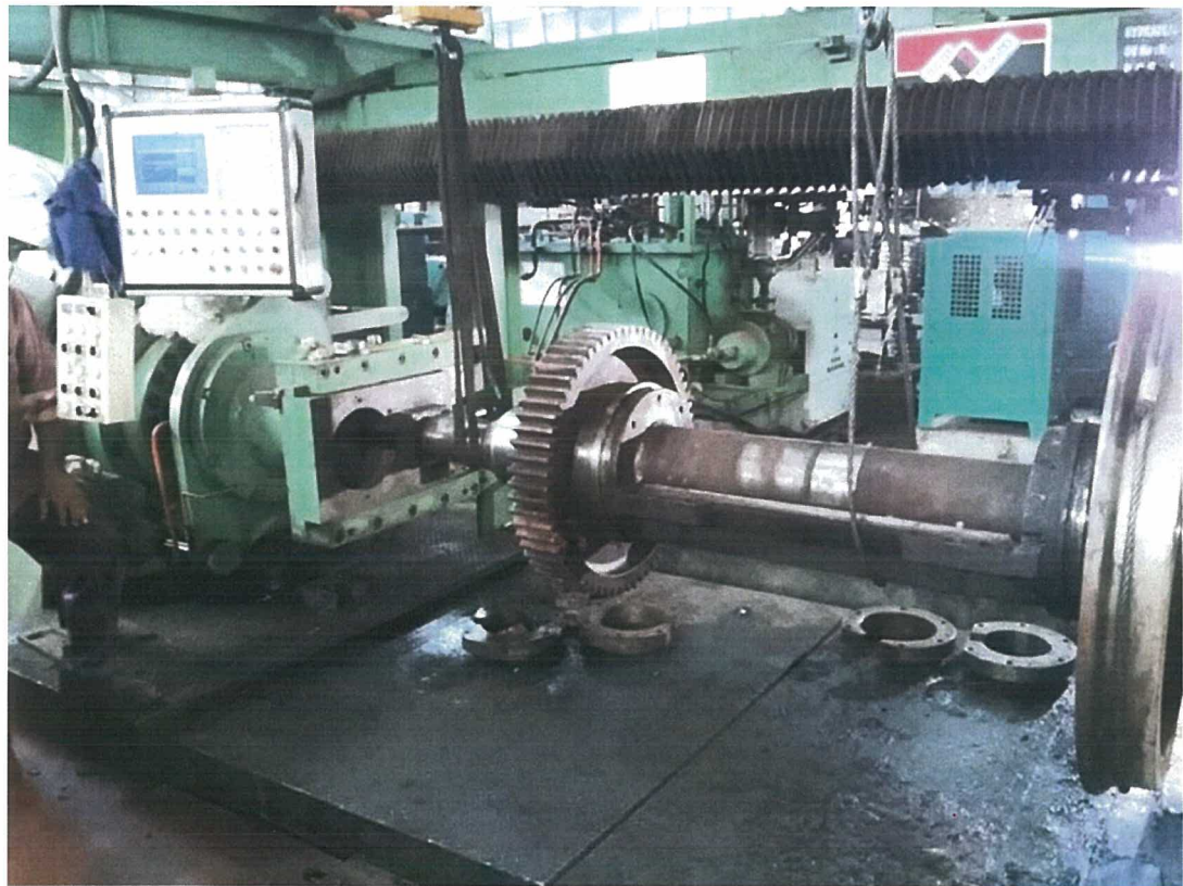
Fig 6 : Wheel disc pressing (Non-Gear Side)
