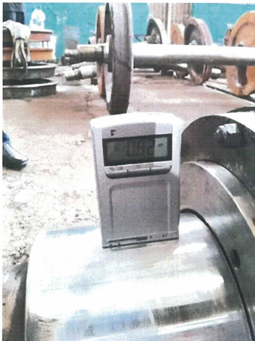
Fig. 5 : Measurement of surface finish of axle at wheel seat
