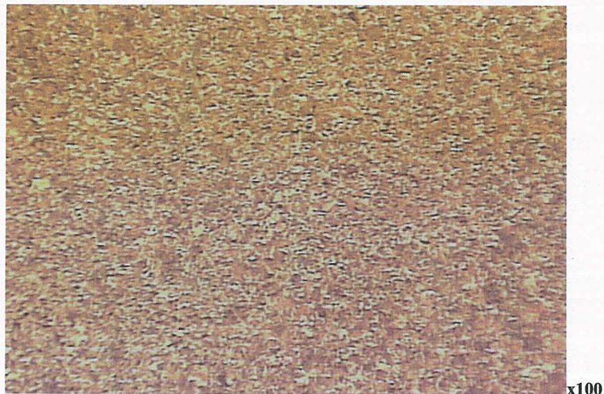
Fig.5 Photomicrograph showing grains of fine pearlite within Thin & broken network of ferrite.
