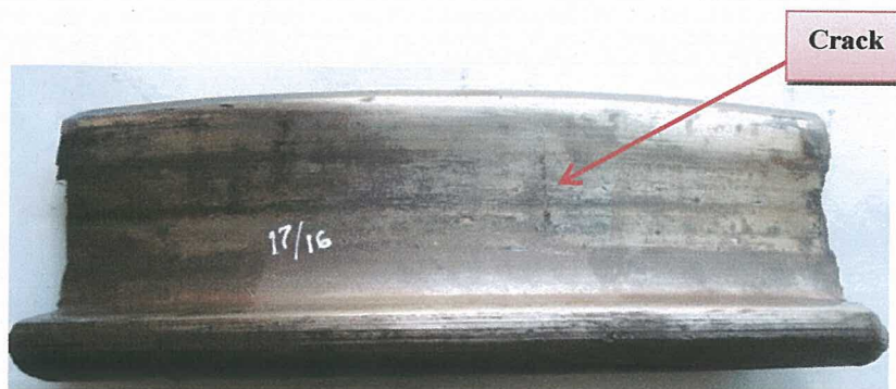
Fig.3 Photograph showing location of crack on wheel tread at corresponding location of fracture initiation zone.
